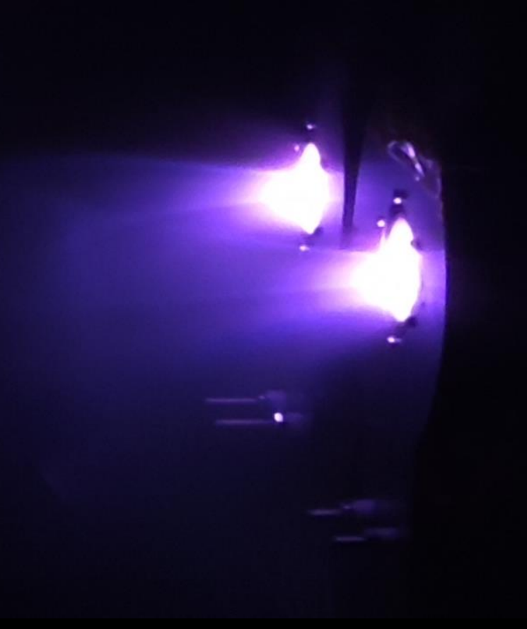
Thruster in operation with Krypton in MFARCH configuration.
