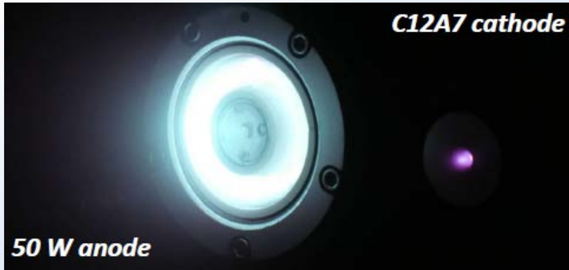
Exotrail hollow cathode coupled with EXOMG-Nano thruster (50 W HET)
