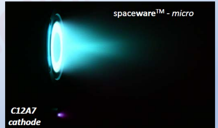
Exotrail hollow cathode coupled with spaceware-micro thruster (150 W HET)
