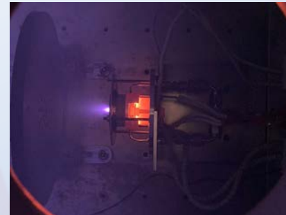
Heated planar insert cathode developed at JLU
