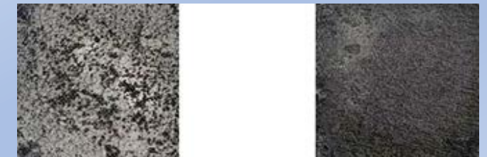
Deposition with binder on carbon fiber (left) and carbon paper (right)
