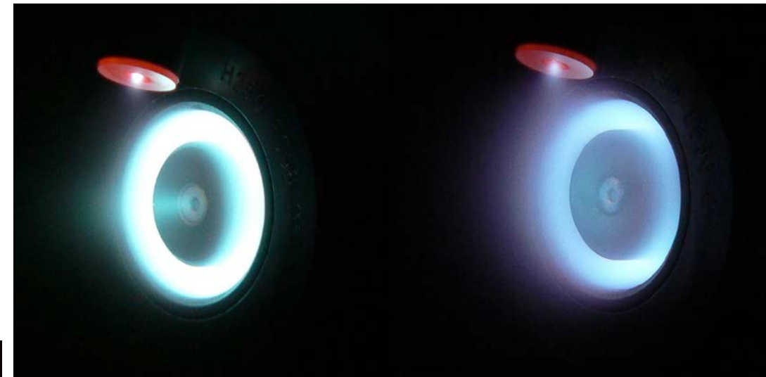
CR HET during firing at high and low power level
