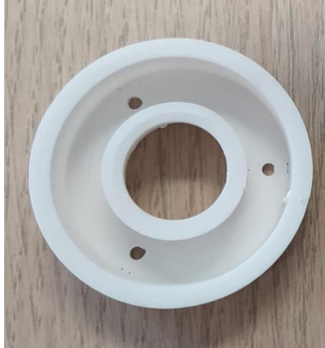
A 3D printed alumina discharge channel for an Hall thruster.
