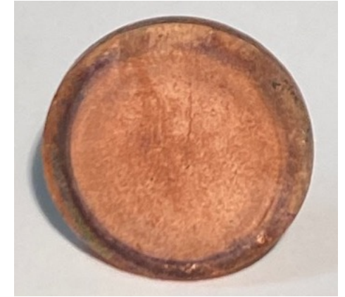
Fig. 8: The inner (negative) electrode of copper after few hours of continuous operation
