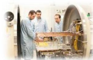
Thermal vacuum - test chamber
